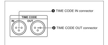
**1 TIME CODE IN connector (XLR 3-pin, female)** To record time code from an external device, input a time code signal from the time code output connector of the other device.
